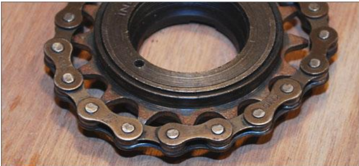
Fig 3.10 This chain is too thin for the teeth [11]
