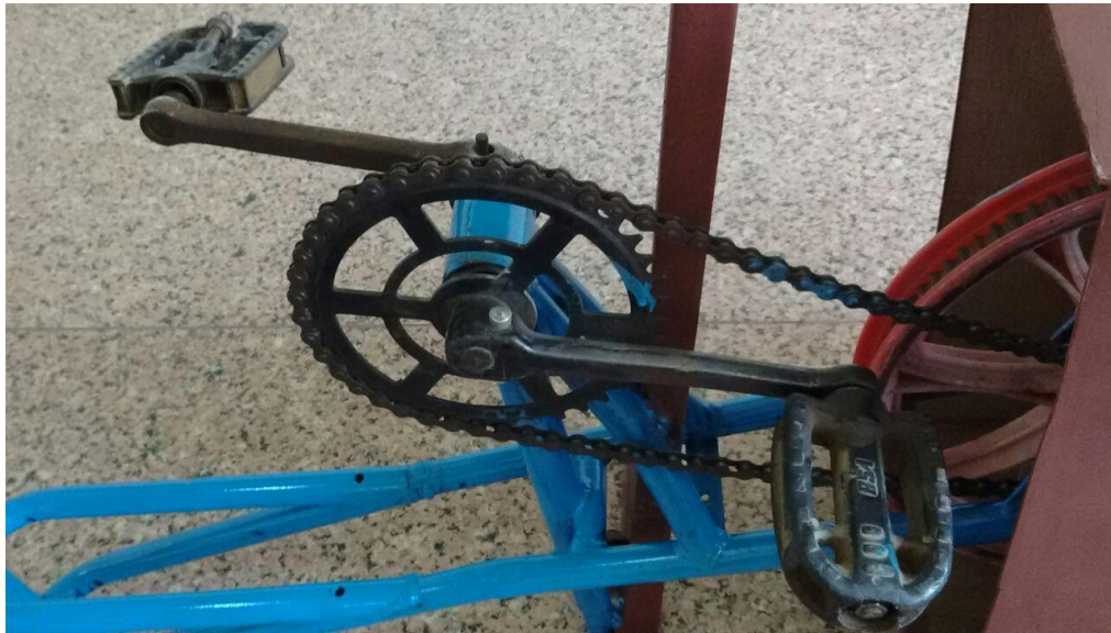
Fig 2.1 Pedal Operated Washing Machine
