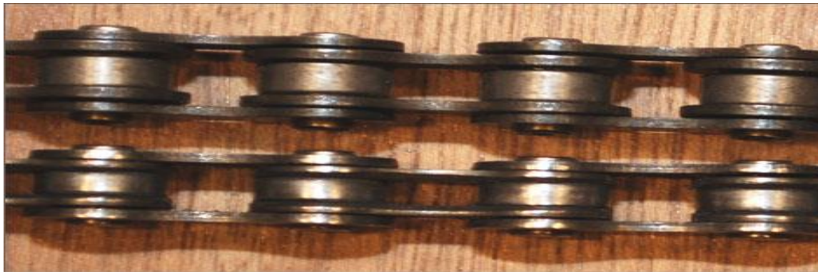
Fig 3.8 Single speed (top) and multi-speed (bottom)[11]
